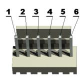
This connector allows programming and debugging via PIC-KIT3 or other compatible tool.
