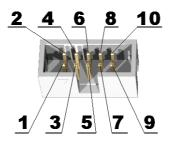
UEXT is connector for external plug-in modules.
