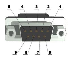
**TXD** Output **Transmit Data.** This is the asynchronous serial data output (RS232) for the shift register on the UART controller.
